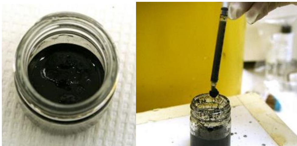
Figure 3. Representative Digital Images of 80-Mesh Crumb Rubber in Ethanol Showing Clumping of Material During Dispensing
