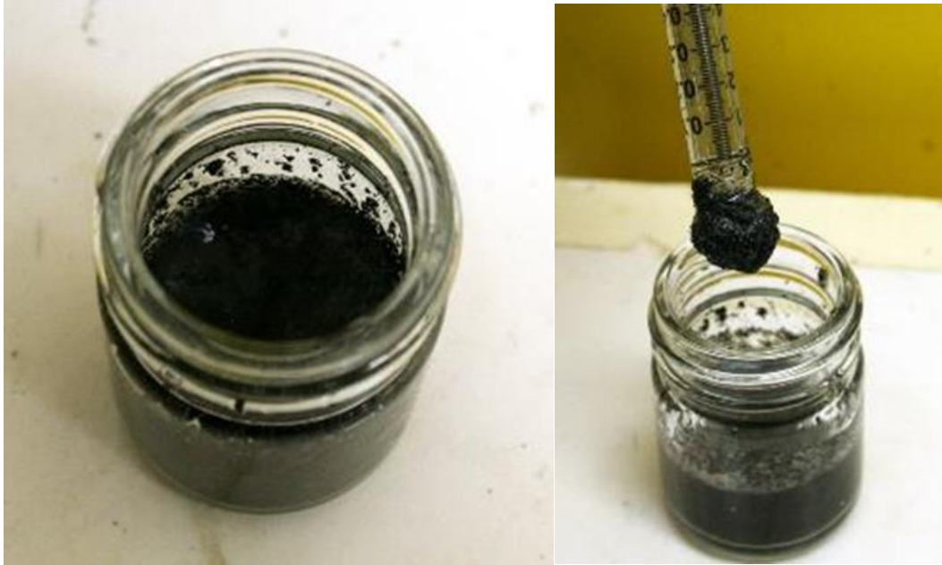
Figure 5. Representative Digital Images of 80-Mesh Crumb Rubber in 0.5% Aqueous Methylcellulose Showing Clumping of Material During Dispensing
