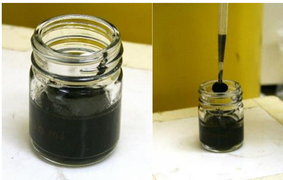
Figure 4. Representative Digital Images of 400-Mesh Crumb Rubber in Ethanol Showing Clumping of Material During Dispensing
