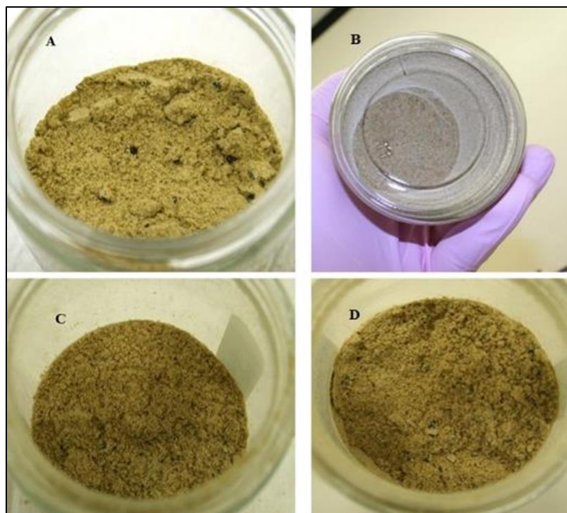
Figure 7. Representative Digital Images of Homogeneity of 14-Mesh Crumb Rubber in Feed Formulation after Shaking on Days 0 (A), 1 (B), 4 (C), and 7 (D)
