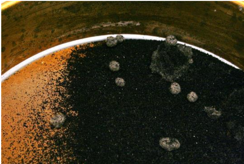
Figure 2. Digital Image of Crumb Rubber at 80-Mesh Particle Size Showing Nylon Bundles
