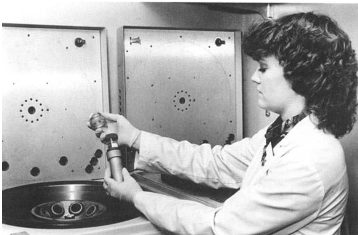
FIGURE 3.2 If a fluid containing an infectious agent were to escape from a centrifuge rotor or cup during high-speed operation, the potential for extensive contamination and multiple infections would be great. The use of sealed buckets, safety trunnion caps, or sealed heads is an effective means of preventing the escape of aerosols. Courtesy, John H. Richardson.
