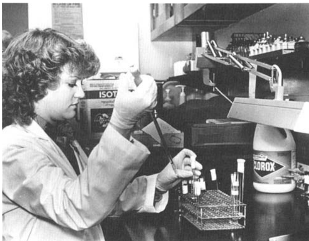
FIGURE 1.1 Do not mouth pipette. Regrettably, many laboratory workers have been taught to pipette by mouth, a practice that has led to a significant number of laboratory-acquired infections. These individuals should be required to give up the old practice and to learn to use the pipetting aids that are now available for any application. Any device requiring mouth suction should be considered unsafe and inappropriate for use in the biological laboratory. Courtesy, John H. Richardson.
