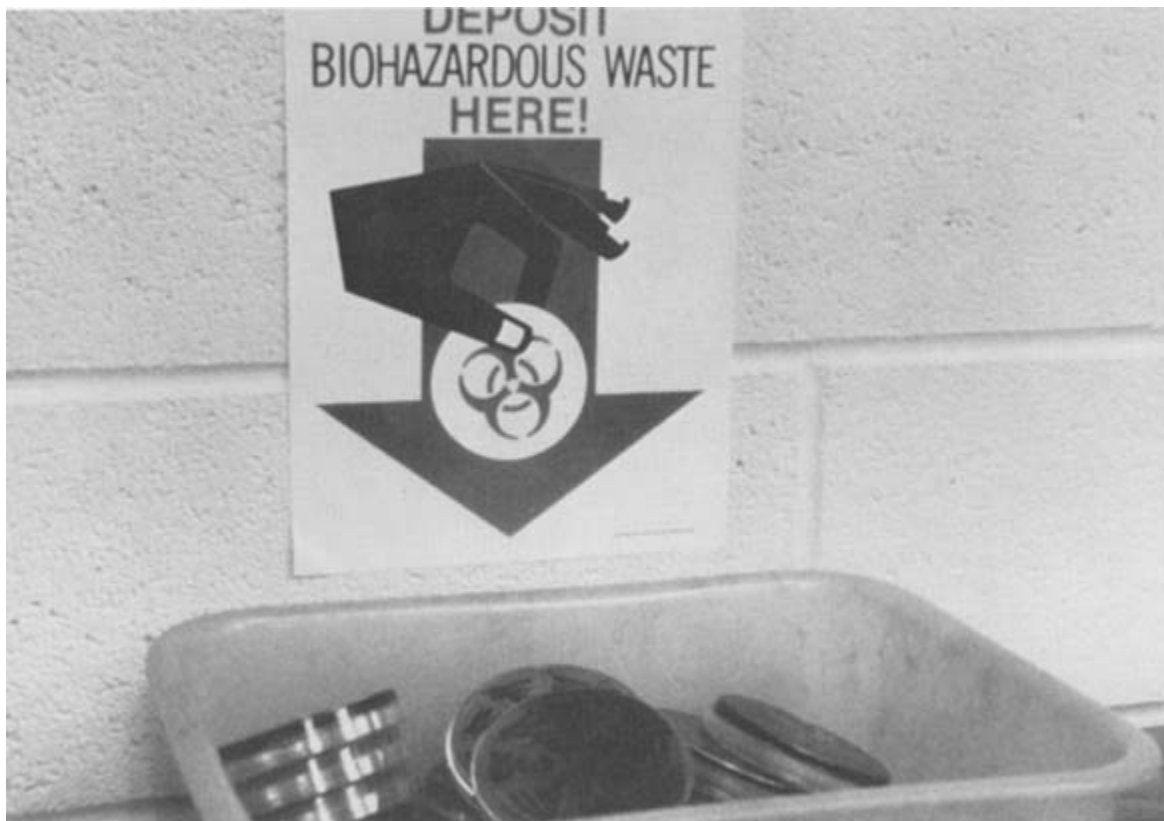
FIGURE 4.1 Biohazardous waste should be segregated from other types of waste prior to its disposal. Courtesy, National Institutes of Health.
