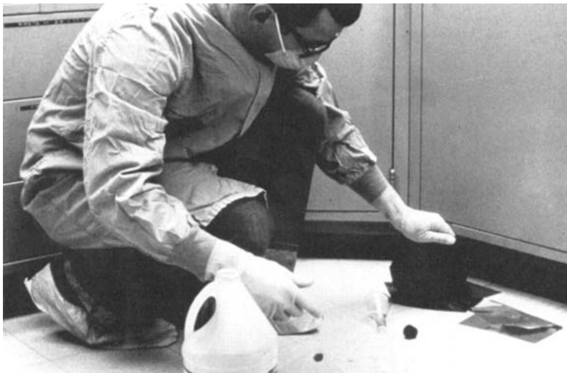
FIGURE 5.1 The cleanup of an accidental spill of biohazardous material is illustrated. A laboratory worker using protective clothing, gloves, and respiratory protection is cleaning up the spill with paper towels that have been soaked with a disinfectant. The proper emergency response for a particular spillage will depend on the volume of the spill and the infectious hazard of the material. Courtesy, National Institutes of Health.
