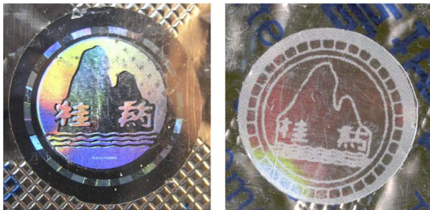
FIGURE 6-10 Genuine (left) and falsified (right) holograms on artesunate blister packs found in Southeast Asia. SOURCE: Newton et al., 2008.
