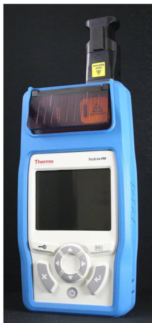
A handheld Raman spectrometer. SOURCE: Zook, 2012.
