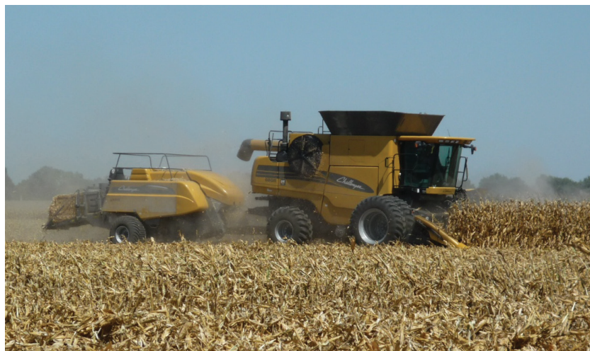
FIGURE 2-4 Single-pass harvest system for corn and corn stover. SOURCE: AGCO Corporation.
