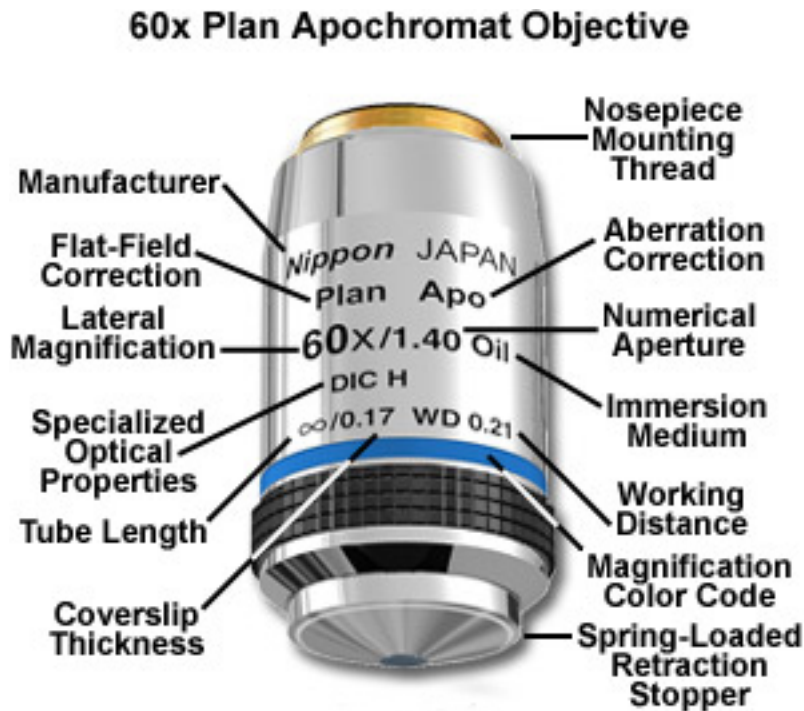
Figure 1: Important properties of objectives are indicated on the barrel of the objective, these include magnification, numerical aperture, working distance, immersion medium and coverslip thickness. Taken from http://www.olympusmicro.com/primer/anatomy/specifications.html
