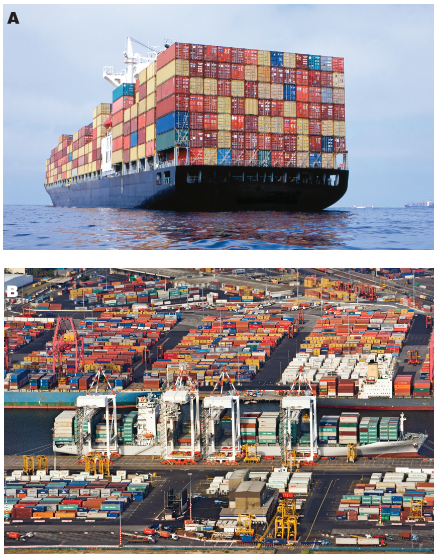
FIGURE 3-5 Containerization. Approximately 90 percent of non-bulk cargo worldwide moves by containers stacked on transport ships. More than 20 million such containers make over 200 million voyages per year; some ships can carry more than 14,500 units. The speed, efficiency, and convenience of this form of transport enable cargoes to be delivered directly from the ship to their destination with minimum delay at the dockside. In consequence, it has become totally impractical to make routine inspections, either at the port of arrival or at the point where the container is finally opened. SOURCE: Fotosearch, LLC.
