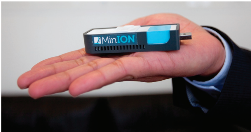
FIGURE WO-46 Prototype of a nanopore sequencing technology currently under development.
